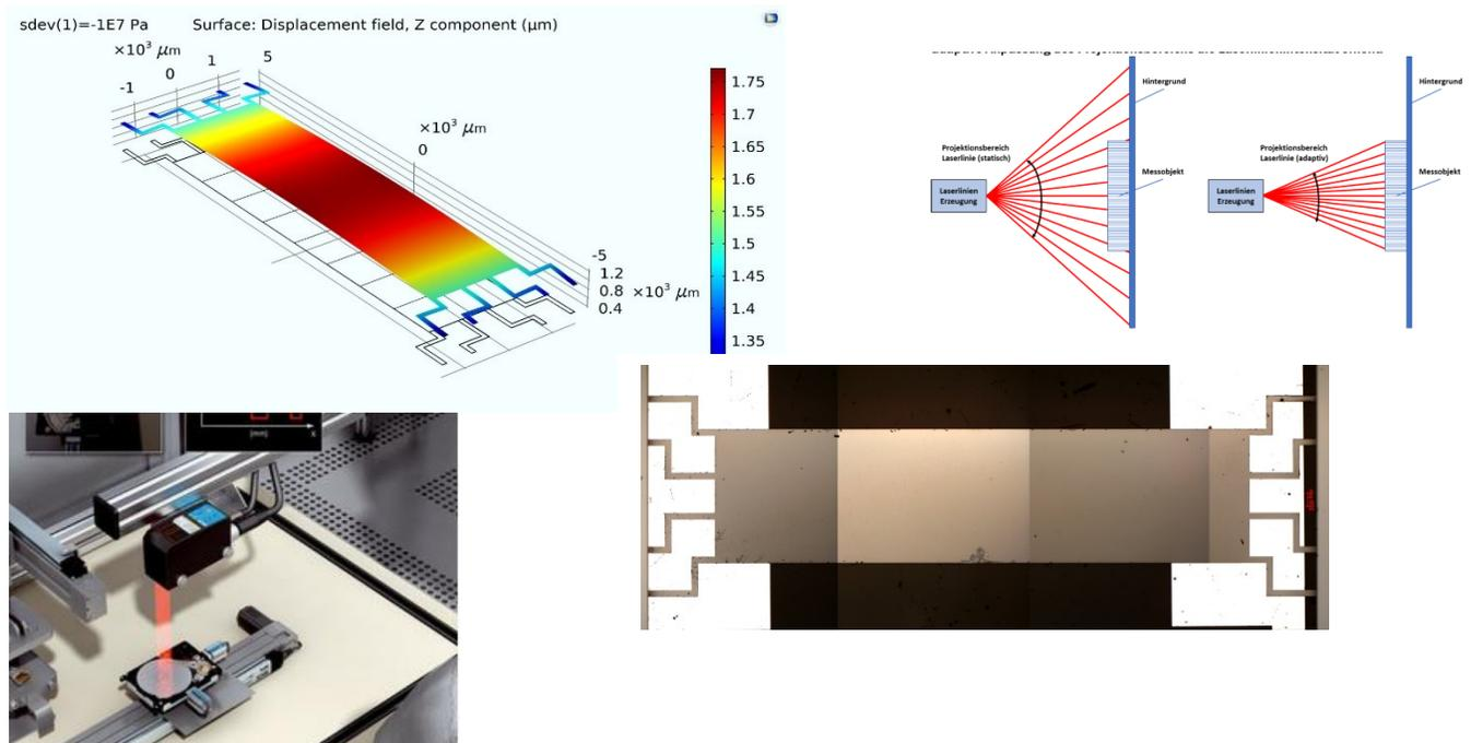
Fig.: Top left: simulated bending of the micromechanical, cylinder shaped membrane, top right: principle of laser beam adjustment, bottom left: Profilometer, Sick AG, bottom right: microscopic picture of fabricated micromechanical device
