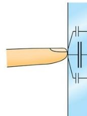
Fig. 2: principle set-up of PCAP [<https://www.adm-electronic.de/blog/technologien/pcap-touch-sensor/>]
