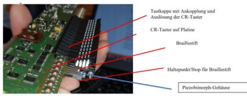
Fig.1 Inside view of Braille display, courtesy S. Kipke Helptech
